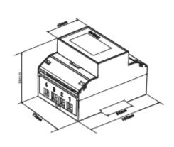
Height 100mm Width 72mm Depth 66mm
